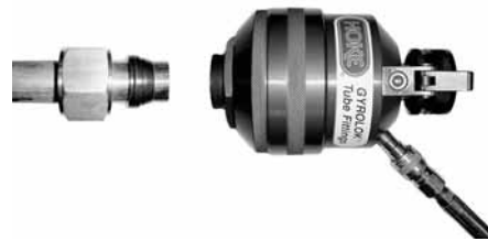
Pre-set tube assembly is ready for installation using standard Gyrolok remake instructions
