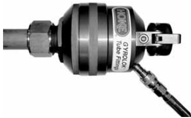
Gyrolok nut and ferrule system components are assembled onto Hydraulic Pre-Setting Tool. Hand pump is operated until indicator arm releases.
