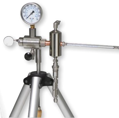
The Model 13 Bureau of Mines Dew Point Tester is a chilled mirror device that operates by achieving the conditions required by the definition of dew point.
